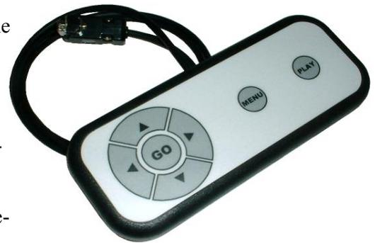
This sensor allows the inserted media to be activated, played, by a passer-by (pedestrian) when used within a kiosk environment where, for example, a DVD player system is used to provide Point-of-Sale (POS) advertising.
