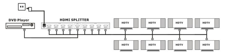
**Note:** When HDMI Splitter works, make sure the source device and display device are well connected with cables. In order to make the relevant ports firstly power on switch, then power on source device.
