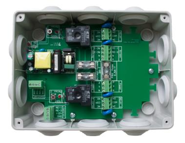
The Impera<sup>™</sup> SR-2 is a two-relay unit designed for simple applications when only minimal switching is required, such as raising and lowering a screen. Control is via dedicated inputs, one for each relay, accepting control signals from an Impera controller. Separate high-voltage relay connections are provided, as well as a dedicated "screen mode" connection. Test buttons are provided for manual activation of relays, with LEDs for indication of relay state (open or pulled).
