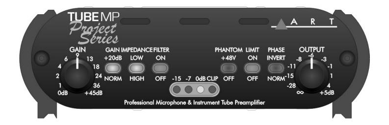
The **Gain** Control directly adjusts the input amplifiers giving you control over the dynamic range of your source. You get a 45dB range of control when using the XLR input and a 25dB range when using the ½" input. Set the control counterclockwise to minimum gain when connecting the inputs.
